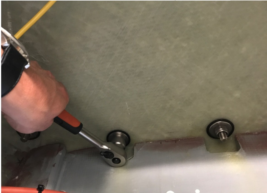
Figure 11 Note metal washers in place before tightening nyloc nuts
