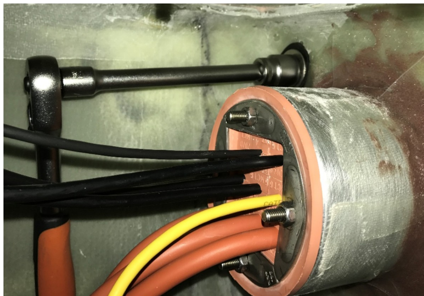
Figure 12 Socket extender required for nut adjacent to hull gland
