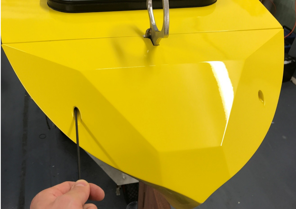
Figure 45 Fixing stern cone into position using long Allen key
