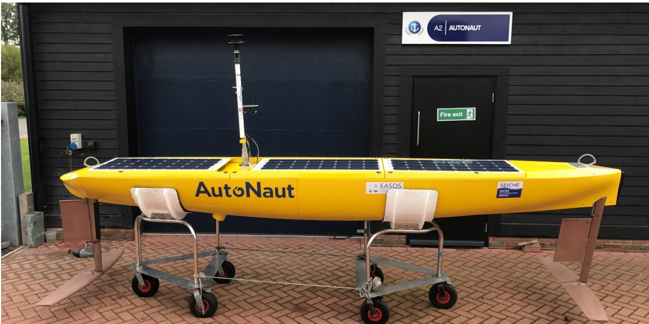
Figure 60 PV panels secured in position. The vessel is ready for launch
