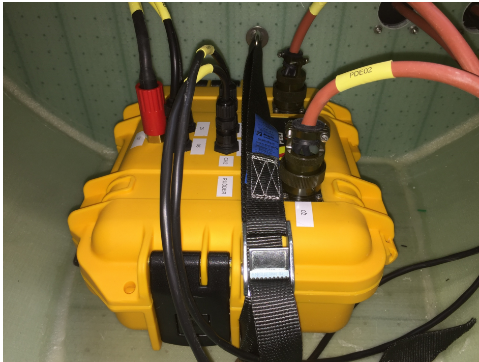
Figure 54 PDE in position and secured
