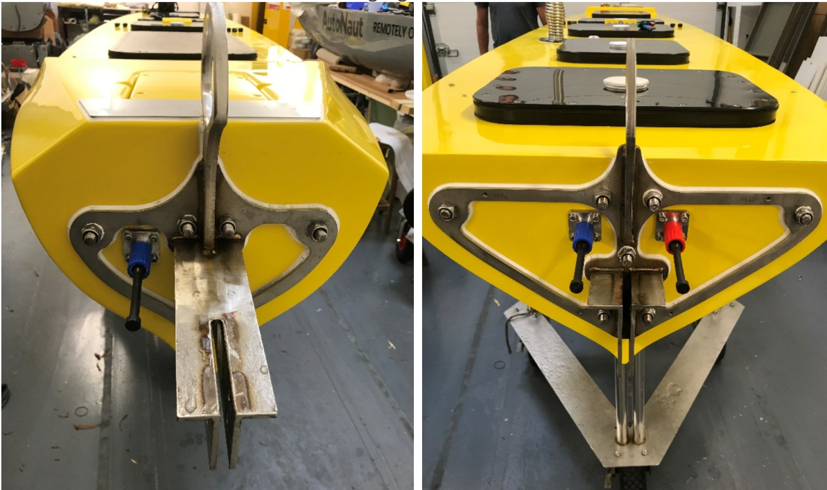
Figure 29 Bow assembly (left) Stern assembly (right) before strut is fitted
