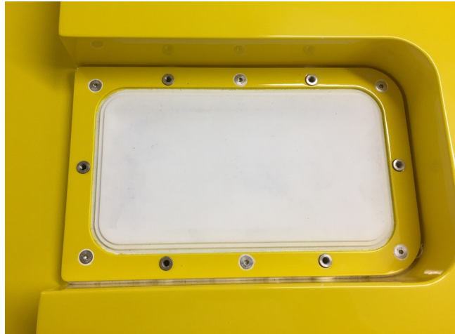
Figure 55 Blank bow connector / key switch plate
