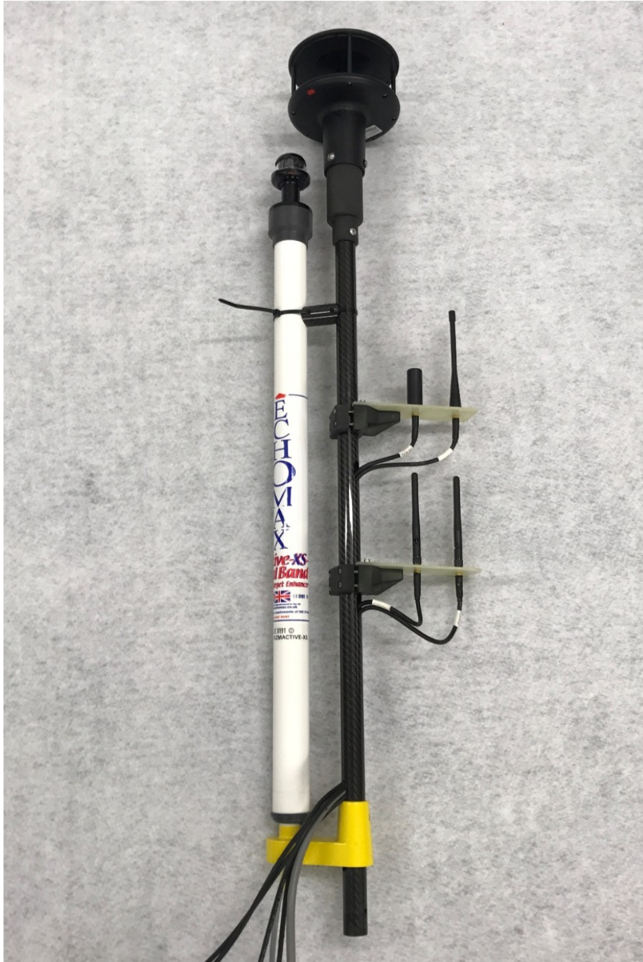
Figure 46 Mast complete with, light and wind sensor
