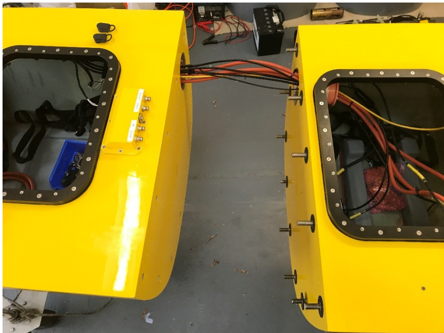
Figure 10 Rubber washers on bolts, cables passed through gland, ready to join hulls
