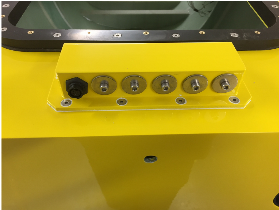
Figure 48 Mast antenna connector box
