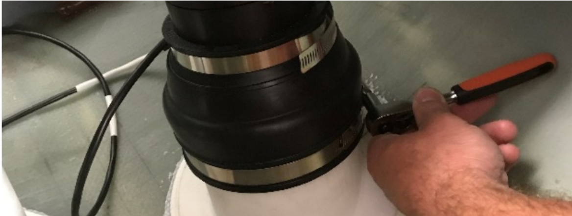
Figure 18 ADCP in position and fitted by tightening jubilee clip on rubber boot around white mount
