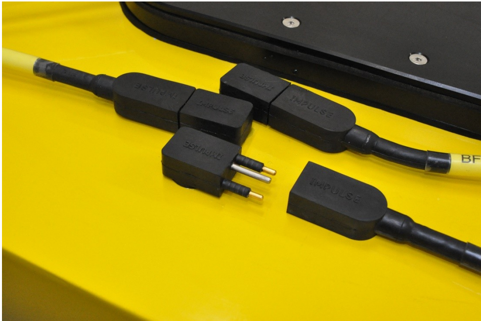
Figure 59 PV panel connectors, 2 are connected, 1 is ready to connect
