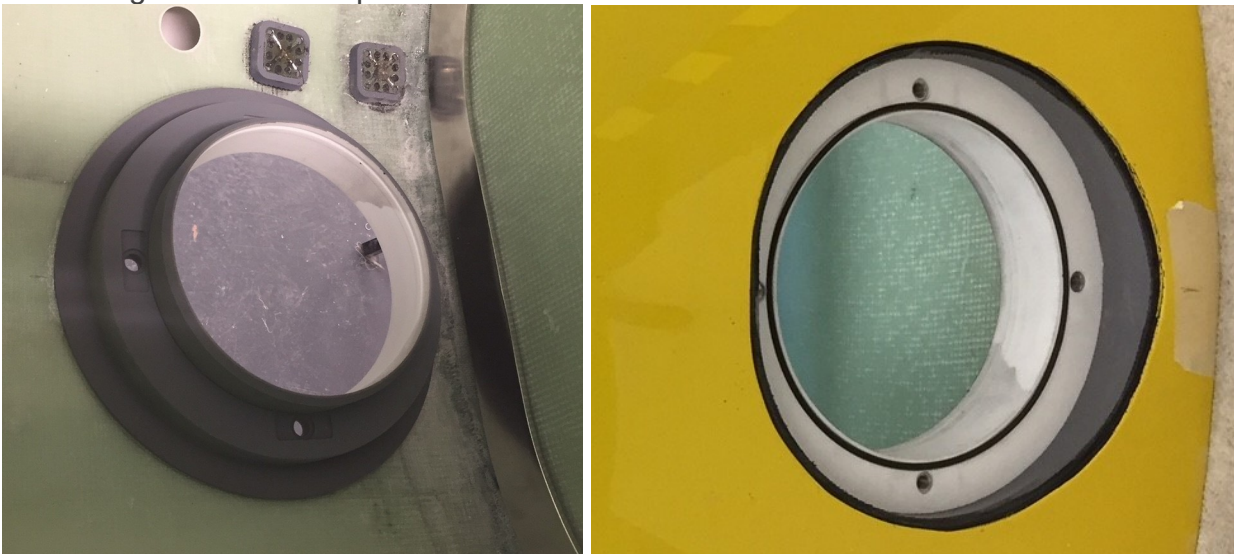
Figure 16 Internal and External images of ADCP mount.
