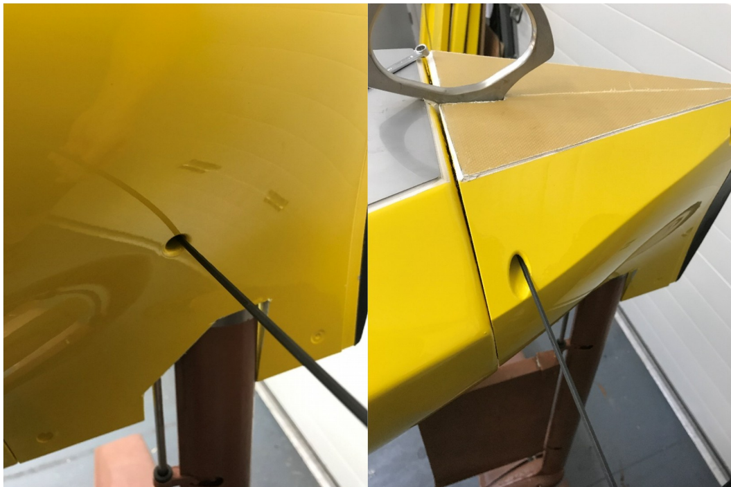
Figure 40 Starboard side bow cone securing in position with Allen key
