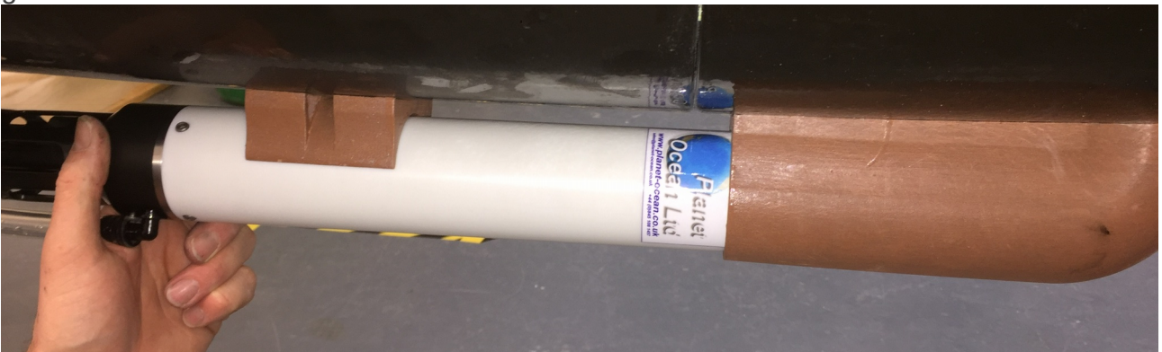
Figure 21 Slide CTD into back bracket
