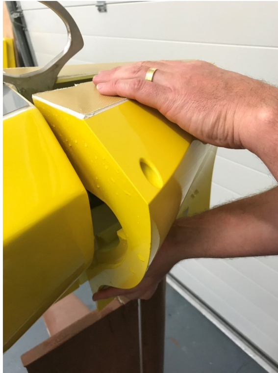
Figure 39 Starboard side bow cone placed into position
