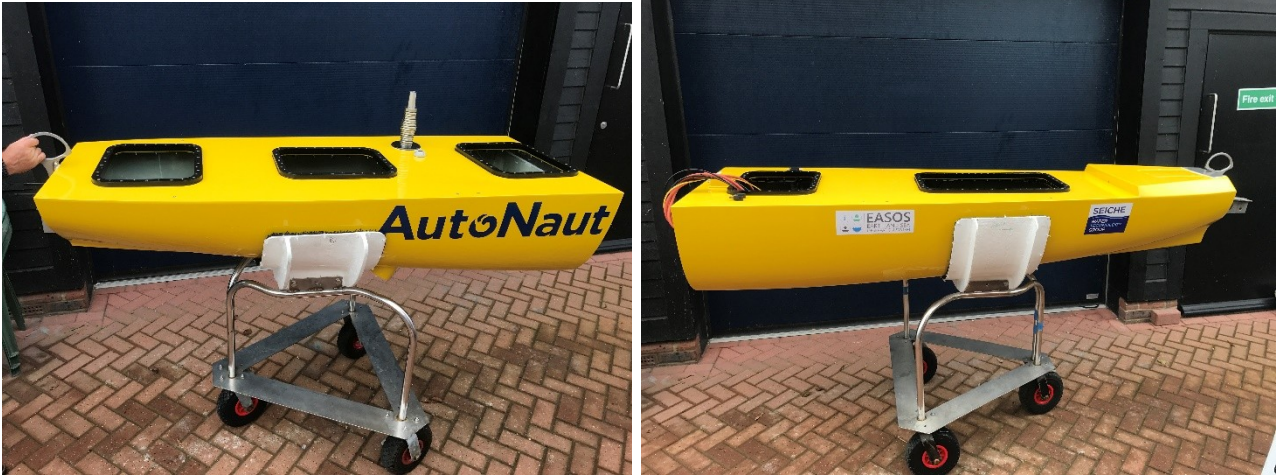
Figure 7 Stern (left) and Bow (Right) hull sections
