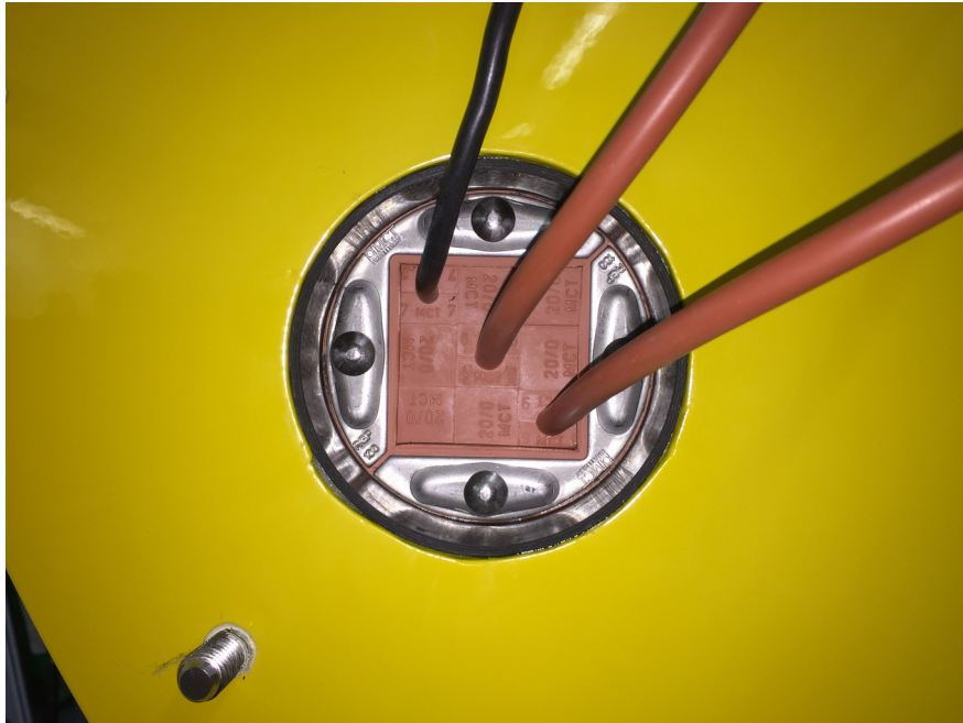
Figure 13 Stern through Gland Cable Layout
