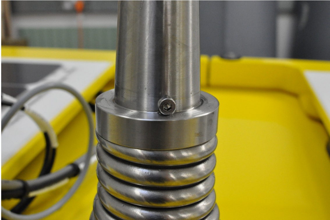
Figure 47 Secure mast into mast base with allen bolts
