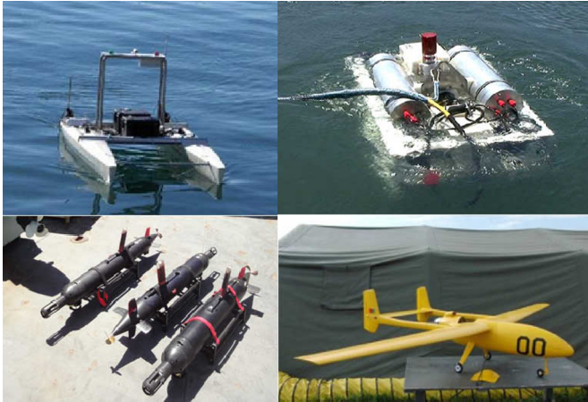
Fig. 2. LSTS autonomous vehicles. From top left to bottom right: Swordfish ASV, Adamastor ROV, LAUV and Antex X03 UAV.
