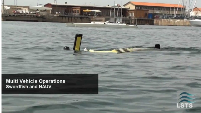
Fig. 9. LSTS nAUV and ASV Swordfish performing cooperative maneuvers.
