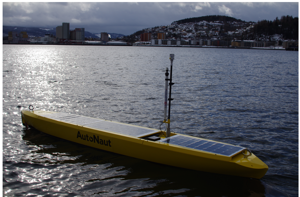
Figure 3. NTNU AutoNaut during operations in Trondheimsfjord.
