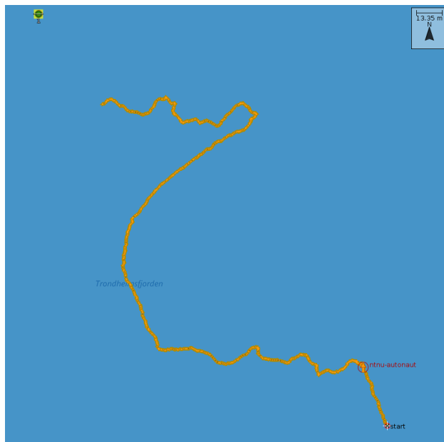
Figure 10.8: AutoNaut maneuvering towards a waypoint position North.
