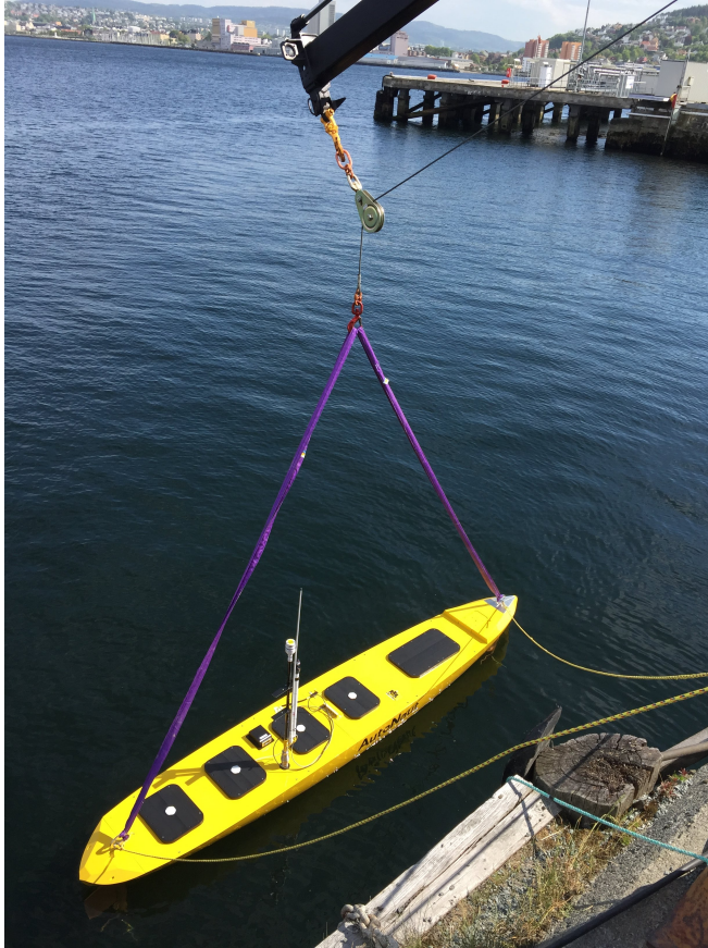
Figure 10.3: Performing rudder, thruster and leakage tests
