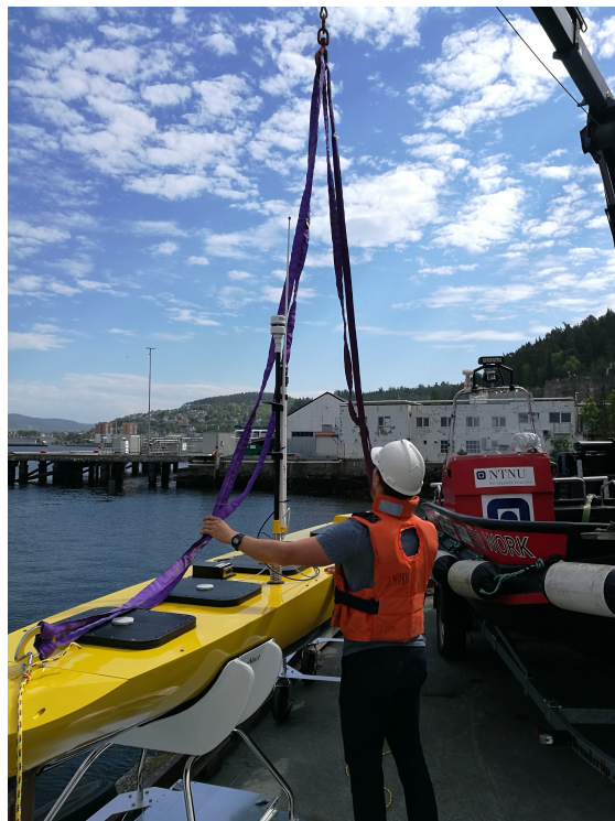
Figure 10.2: The procedure of moving AutoNaut in/out of the water.
