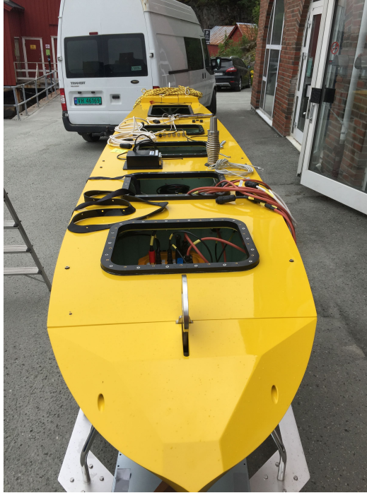
Figure 10.1: Assembling AutoNaut and fitting the sensors
