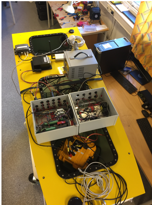
Figure 9.2: Hardware testing of Level1 and Level2 with the rudder and thruster, prior the land-based test
